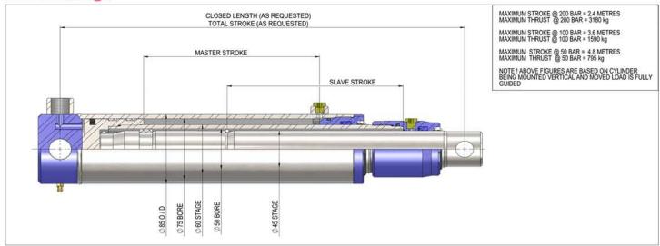
Constant velocity telescopic cylinders are designed to extend and retract at a constant speed and are ideal for applications such as elevators, platform lifts and crop sprayers.
